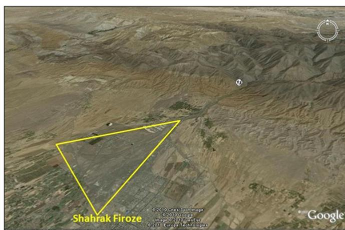
**Figure 3:** Location of Shahrake Firouzeh Site relative to alluvial fan.
